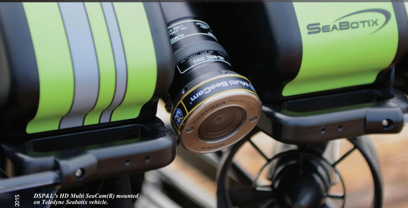
DSP&L's HD Multi SeaCam(R) mounted on Teledyne Seabotix vehicle.
